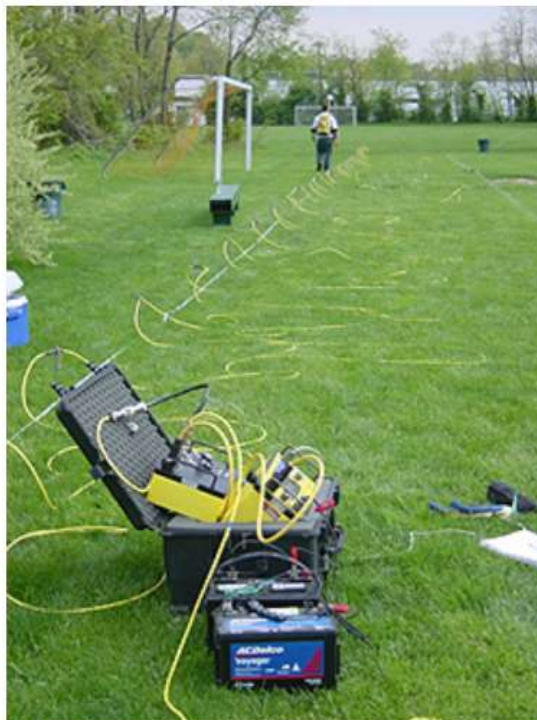
Figure 4.2 This image displays the correct operational setup using the SuperSting resistivity meter, Swift switch box, and 12V battery connected to the multiconductor cables and steel electrodes. Photo retrieved from Advanced Geosciences Inc (2017).
