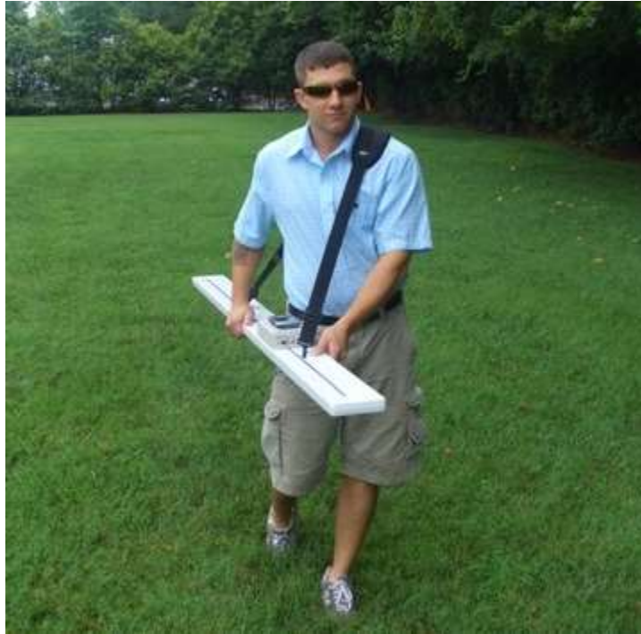
Figure 5.1: Geophex GEM-2 Ski Demonstration, Courtesy of Geophex Ltd.
